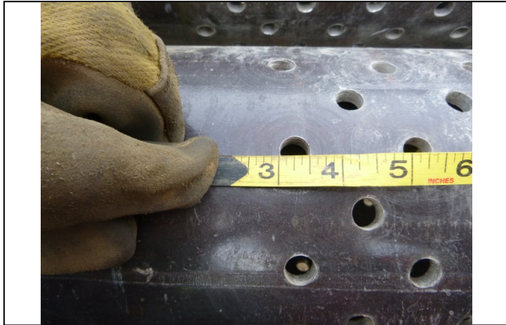
PHOTO 1 – Variperperm 9.4% perforated pipe screen section
