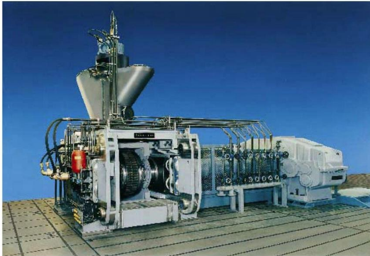
Figure 2: Briquetting machine for DRI from pellets and lump ore, roller diameter 1,000 mm
