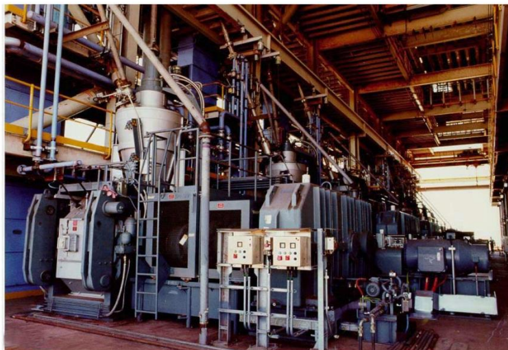
Figure 3: Briquetting machine for the production of HBI from fine ore, roller diameter 1,400 mm
