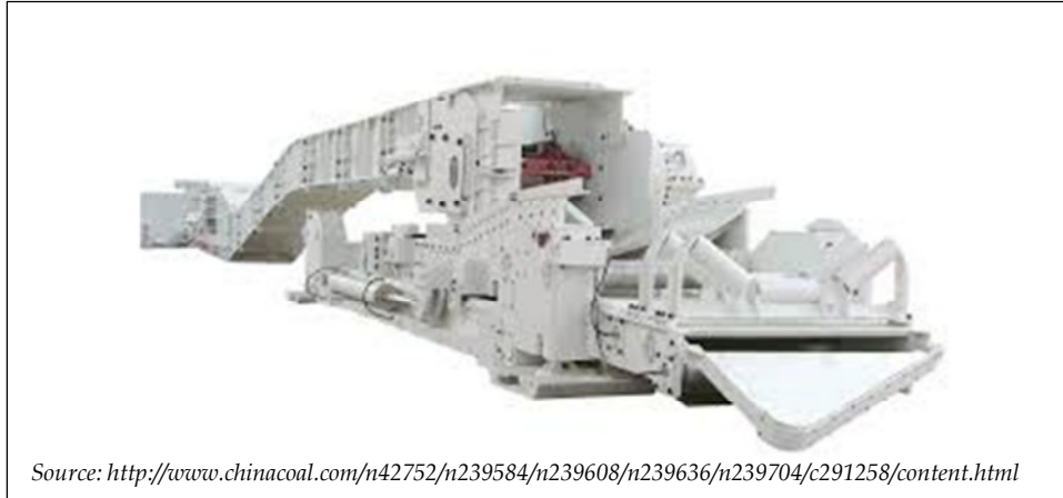
Plate 3.6-4. Beam stage loader.
