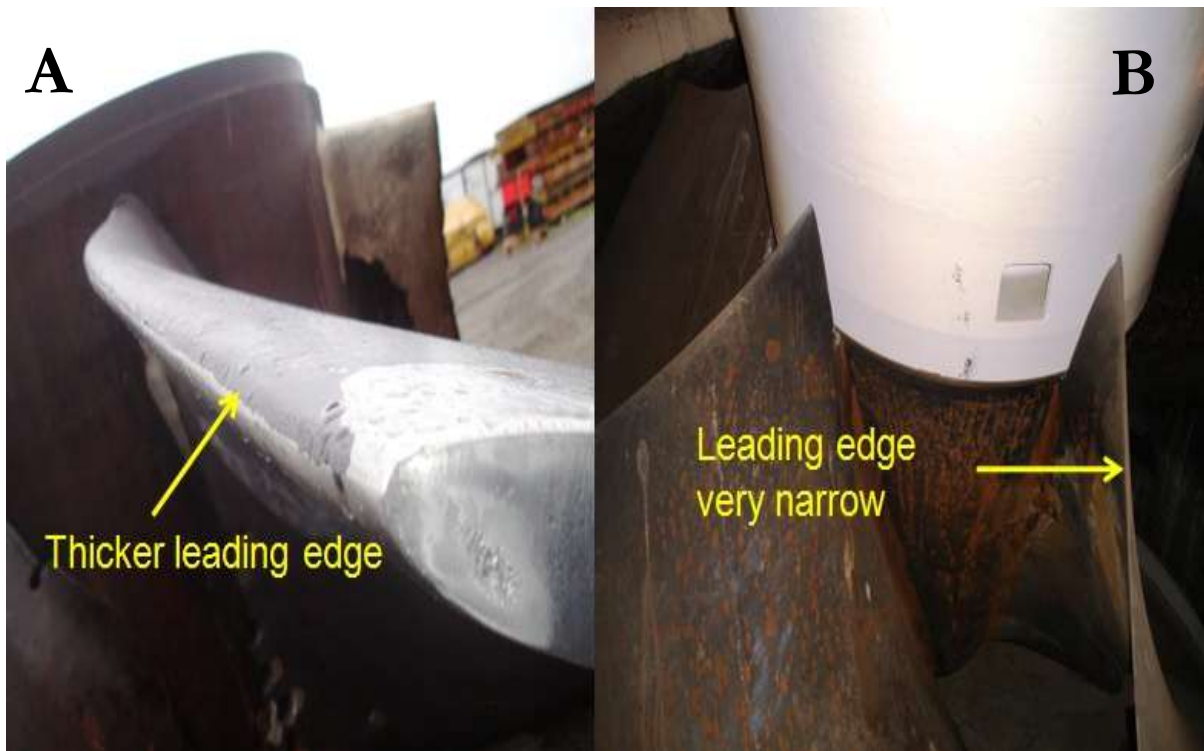
Figure 1: Comparison of leading edge shape and thickness of blades for a 6 (A) and 5 (B) bladed turbine at Manitoba Hydro's Kelsey Generating Station
